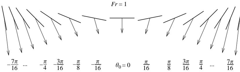
FIGURE 3. The initial force vector on a falling plate after release from rest at modified Froude number  $Fr = 1$ . The vectors shown represent the initial force on the plate's centre of mass (normalized so that the magnitude of the longest vector is 3) for the initial angles  $\theta_0 = -7\pi/16, -3\pi/8, -5\pi/16, \dots, 5\pi/16, 3\pi/8, \text{ and } 7\pi/16$ .
