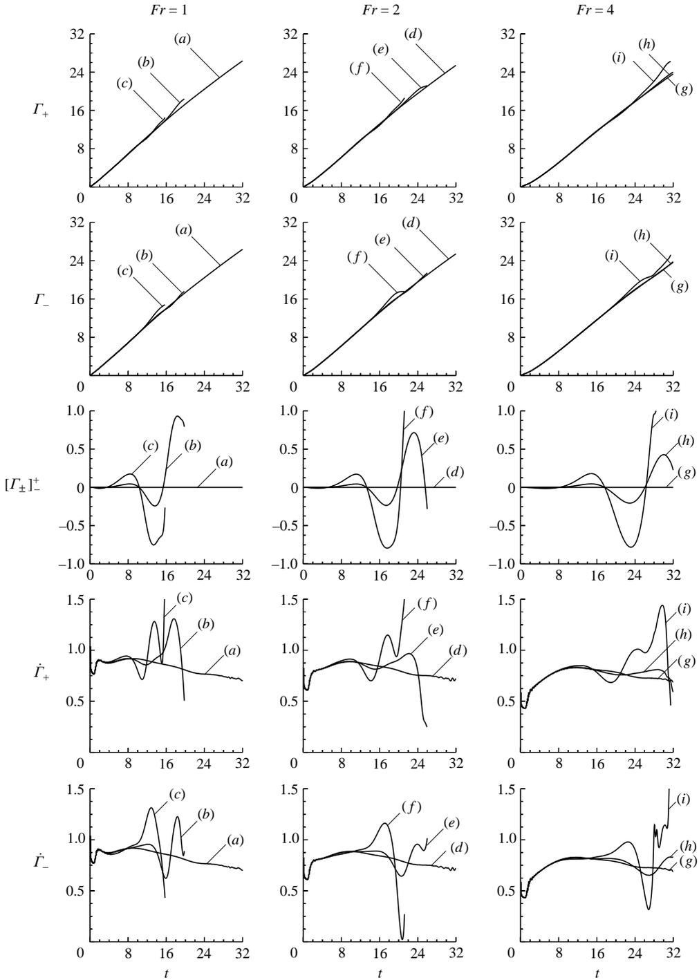
FIGURE 13. The circulation around a falling plate after release from rest; examples (a)–(i). The functions  $\Gamma_+(t)$  and  $\Gamma_-(t)$ , the bound circulation  $[\Gamma_{\pm}(t)]_{\pm}$ , and the shedding rates  $\dot{\Gamma}_+(t)$ , and  $\dot{\Gamma}_-(t)$  are plotted for modified Froude numbers (a)–(c)  $Fr = 1$ , (d)–(f)  $Fr = 2$ , and (g)–(i)  $Fr = 4$  and initial angles (a)(d)(g)  $\theta_0 = 0$ , (b)(e)(h)  $\theta_0 = \pi/1024$ , and (c)(f)(i)  $\theta_0 = \pi/256$ .
