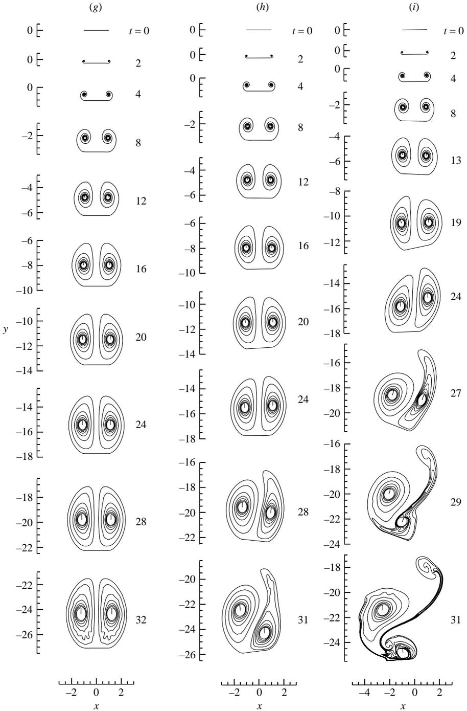
FIGURE 12. Examples (g), (h), and (i). The trailing vortex sheets left behind a falling flat plate with  $Fr = 4$ . The wake is visualized at times  $t = 0, 2, 4, 8, 12, 16, 20, 24, 28$ , and  $32$  for (g)  $\theta_0 = 0$ . At times  $t = 0, 2, 4, 8, 12, 16, 20, 24, 28$ , and  $31$  for (h)  $\theta_0 = \pi/1024$ . And at times  $t = 0, 2, 4, 8, 13, 19, 24, 27, 29$ , and  $31$  for (i)  $\theta_0 = \pi/256$ .
