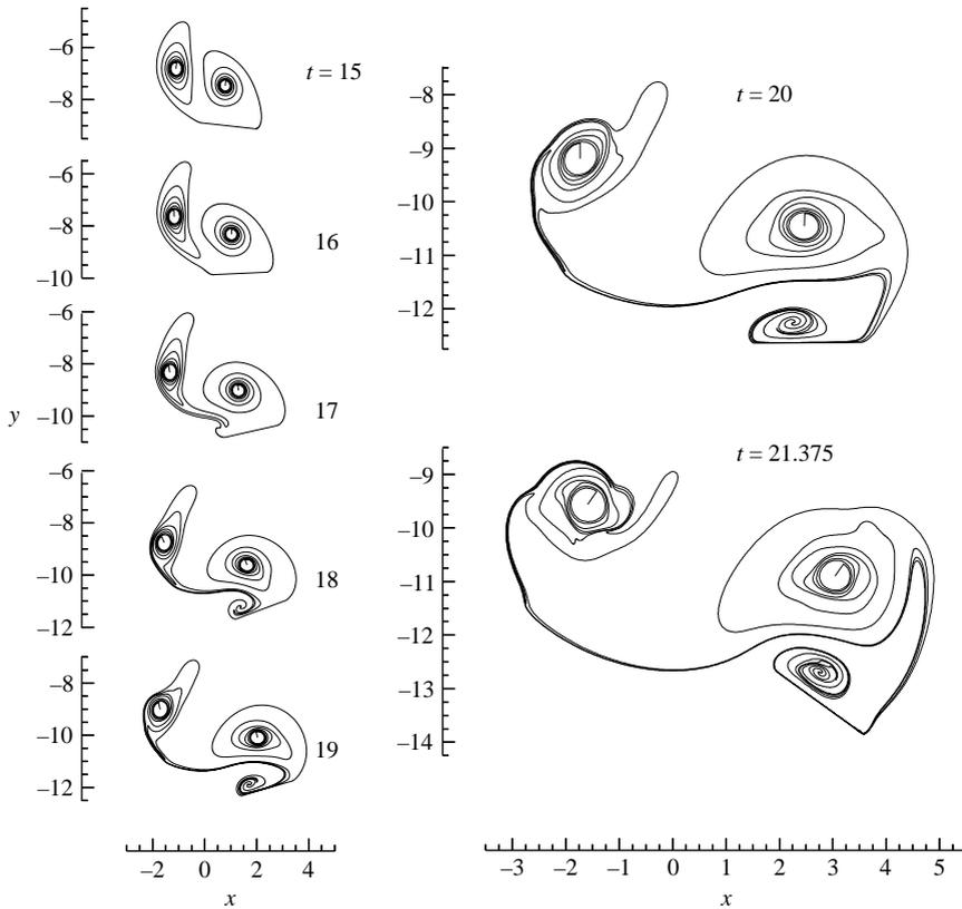
FIGURE 15. Example (j). The trailing vortex sheets left behind a falling flat plate with  $Fr = 4$  and  $\theta_0 = \pi/32$ . The wake is visualized at times  $t = 15, 16, 17, 18, 19, 20$ , and  $21.375$ ; the frames for  $t = 20$  and  $21.375$  are shown magnified by a factor of 2.
