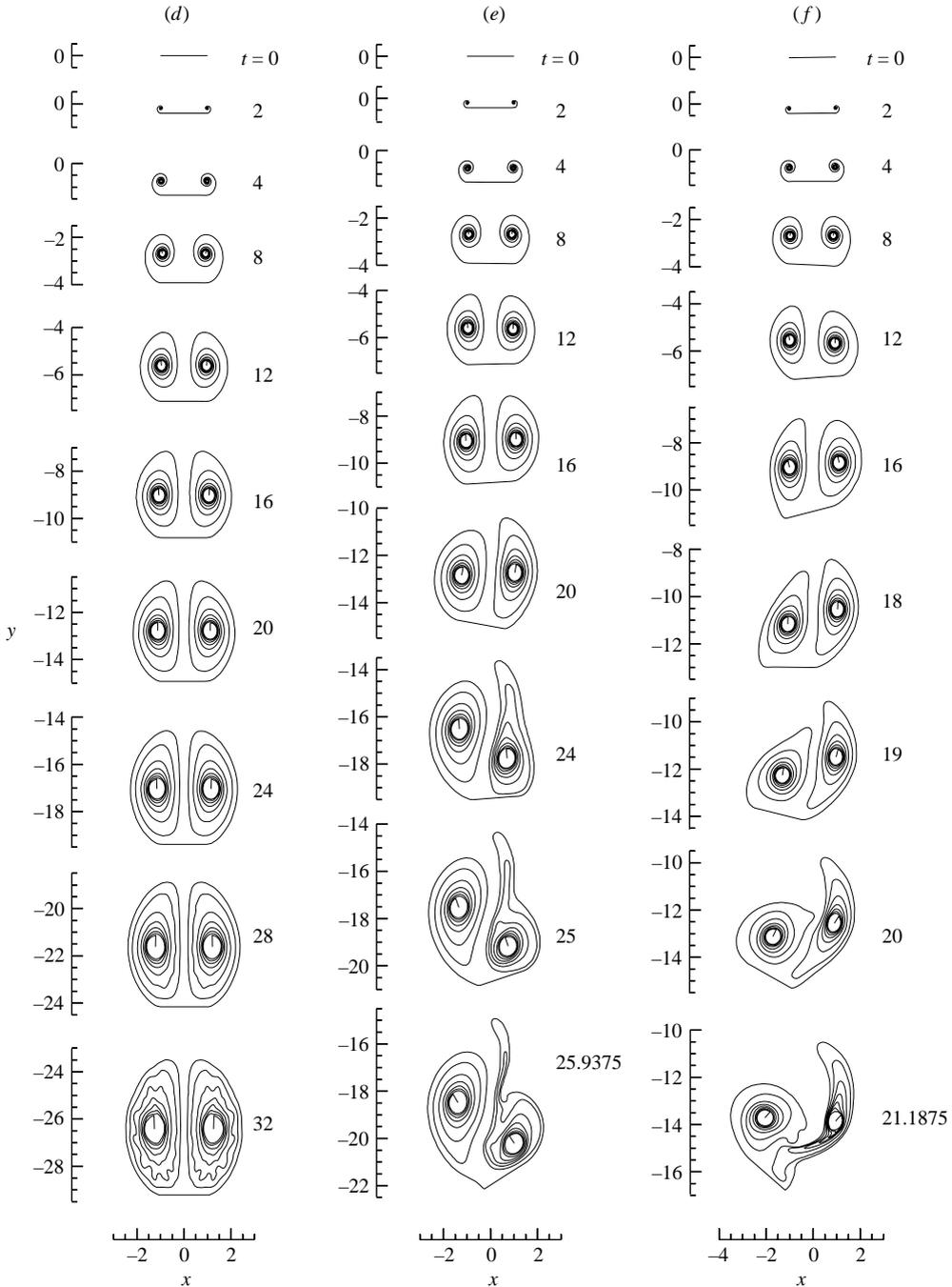
FIGURE 11. Examples (d), (e), and (f). The trailing vortex sheets left behind a falling flat plate with  $Fr = 2$ . The wake is visualized at times  $t = 0, 2, 4, 8, 12, 16, 20, 24, 28,$  and  $32$  for (d)  $\theta_0 = 0$ . At times  $t = 0, 2, 4, 8, 12, 16, 20, 24, 25,$  and  $25.9375$  for (e)  $\theta_0 = \pi/1024$ . And at times  $t = 0, 2, 4, 8, 12, 16, 18, 19, 20,$  and  $21.1875$  for (f)  $\theta_0 = \pi/256$ .
