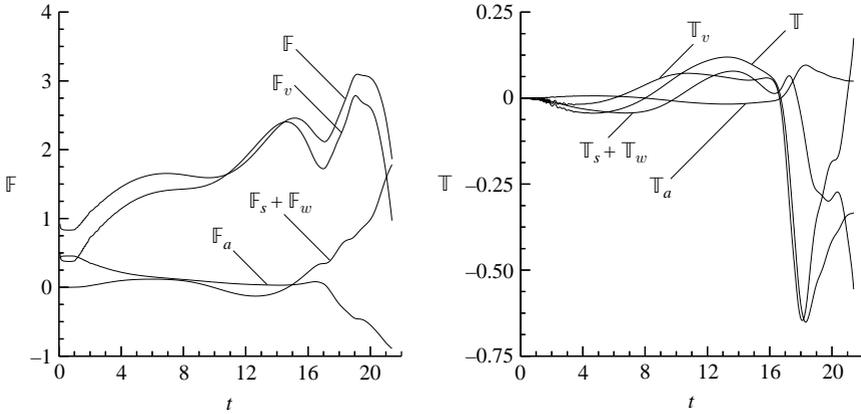
FIGURE 16. Example (j). The total aerodynamic normal force  $\mathbb{F}(t)$  and torque  $\mathbb{T}(t)$  on a falling flat plate after release from rest with  $Fr = 4$  and  $\theta_0 = \pi/32$ . Also plotted, are the corresponding acceleration reactions  $\mathbb{F}_a(t)$  and  $\mathbb{T}_a(t)$ , unsteady vortical contributions  $\mathbb{F}_v(t)$  and  $\mathbb{T}_v(t)$ , and quasi-steady contributions  $\mathbb{F}_s(t) + \mathbb{F}_w(t)$  and  $\mathbb{T}_s(t) + \mathbb{T}_w(t)$ .
