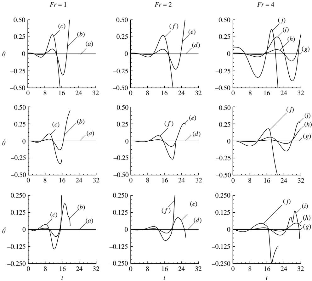
FIGURE 9. The motion of a falling plate after release from rest; examples (a)–(j). The functions  $\theta(t)$ ,  $\dot{\theta}(t)$ , and  $\ddot{\theta}(t)$  are plotted for modified Froude numbers (a)–(c)  $Fr = 1$ , (d)–(f)  $Fr = 2$ , and (g)–(j)  $Fr = 4$  and initial angles (a)(d)(g)  $\theta_0 = 0$ , (b)(e)(h)  $\theta_0 = \pi/1024$ , (c)(f)(i)  $\theta_0 = \pi/256$ , and (j)  $\theta_0 = \pi/32$ .
