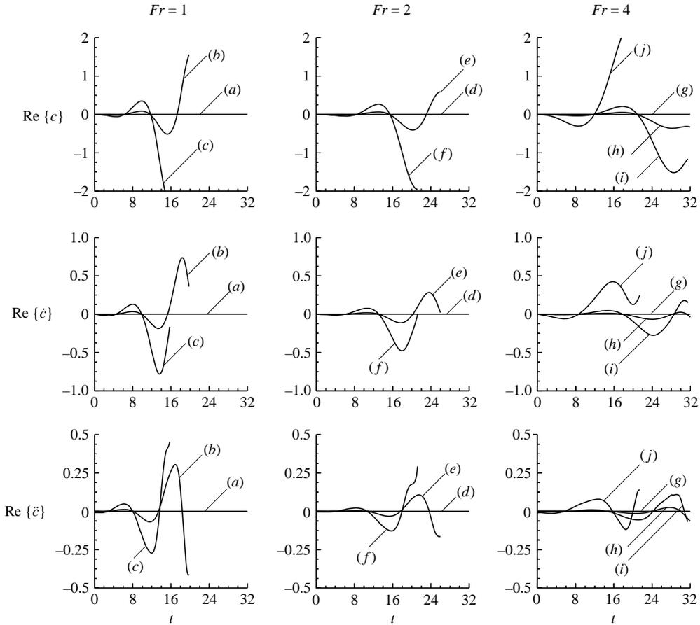
FIGURE 7. The motion of a falling plate after release from rest; examples (a)–(j). The functions  $\text{Re}\{c(t)\}$ ,  $\text{Re}\{\dot{c}(t)\}$ , and  $\text{Re}\{\ddot{c}(t)\}$  are plotted for modified Froude numbers (a)–(c)  $Fr = 1$ , (d)–(f)  $Fr = 2$ , and (g)–(j)  $Fr = 4$  and initial angles (a)(d)(g)  $\theta_0 = 0$ , (b)(e)(h)  $\theta_0 = \pi/1024$ , (c)(f)(i)  $\theta_0 = \pi/256$ , and (j)  $\theta_0 = \pi/32$ .
