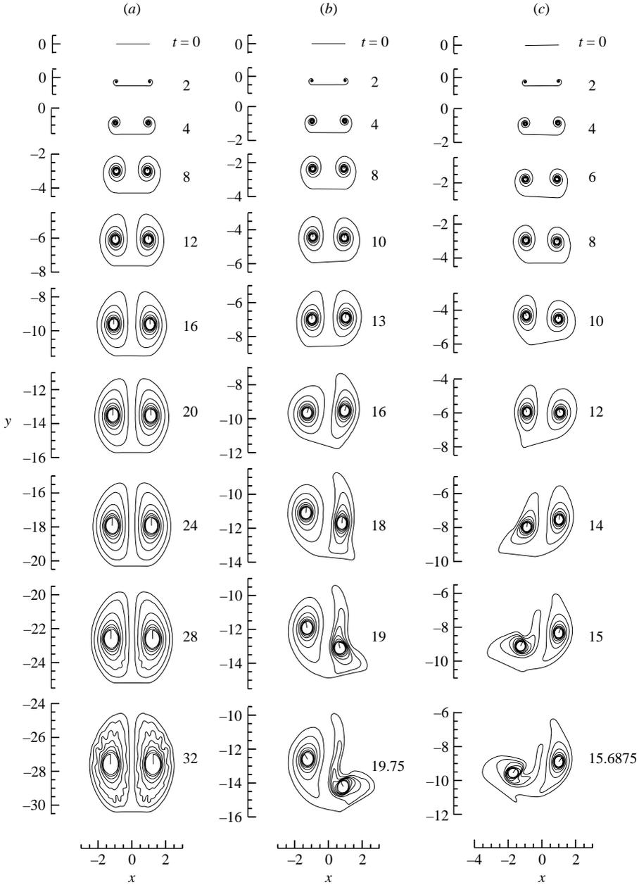
FIGURE 10. Examples (a), (b), and (c). The trailing vortex sheets left behind a falling flat plate with  $Fr = 1$ . The wake is visualized at times  $t = 0, 2, 4, 8, 12, 16, 20, 24, 28$ , and  $32$  for (a)  $\theta_0 = 0$ . At times  $t = 0, 2, 4, 8, 10, 13, 16, 18, 19$ , and  $19.75$  for (b)  $\theta_0 = \pi/1024$ . And at times  $t = 0, 2, 4, 6, 8, 10, 12, 14, 15$ , and  $15.6875$  for (c)  $\theta_0 = \pi/256$ .
