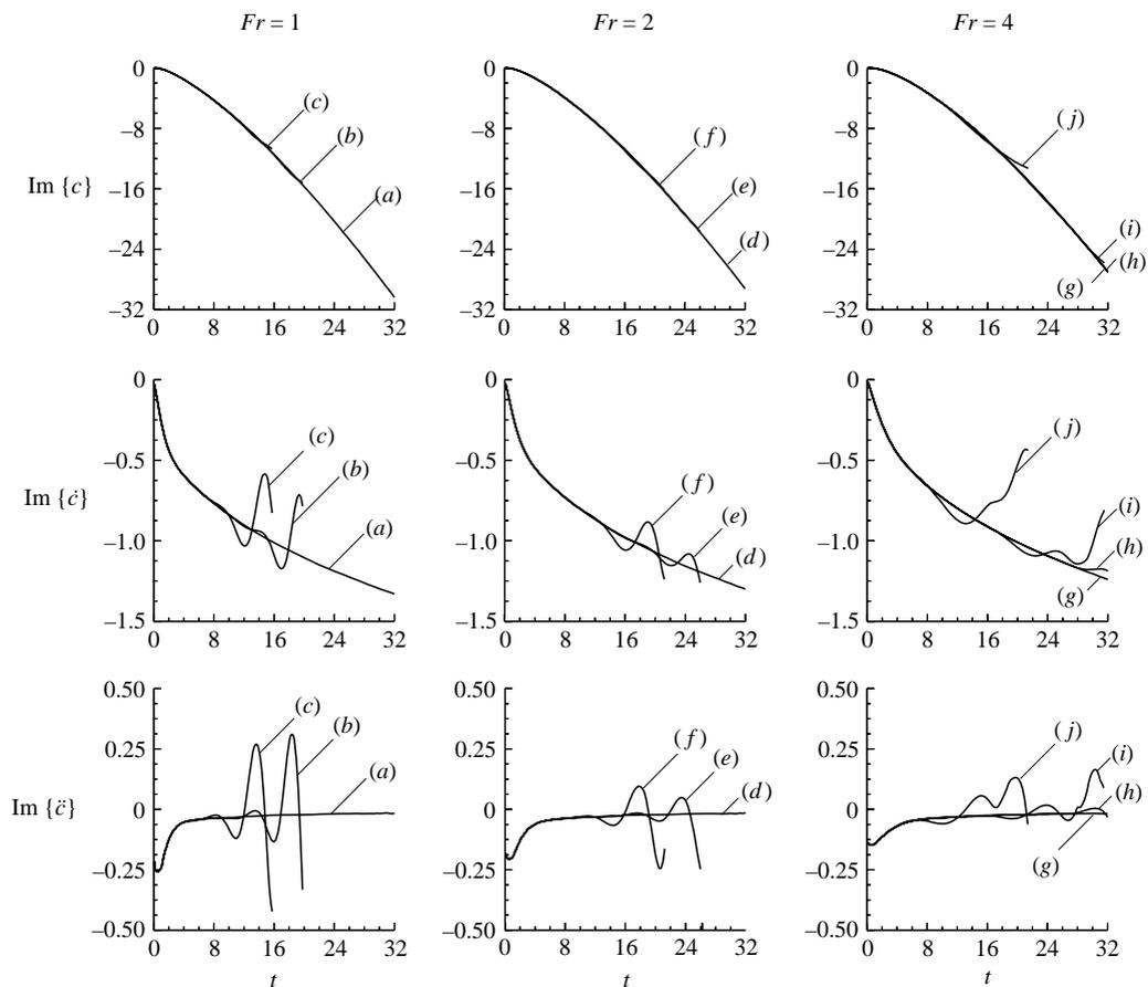
FIGURE 8. The motion of a falling plate after release from rest; examples (a)–(j). The functions  $\text{Im}\{c(t)\}$ ,  $\text{Im}\{\dot{c}(t)\}$ , and  $\text{Im}\{\ddot{c}(t)\}$  are plotted for modified Froude numbers (a)–(c)  $Fr = 1$ , (d)–(f)  $Fr = 2$ , and (g)–(j)  $Fr = 4$  and initial angles (a)(d)(g)  $\theta_0 = 0$ , (b)(e)(h)  $\theta_0 = \pi/1024$ , (c)(f)(i)  $\theta_0 = \pi/256$ , and (j)  $\theta_0 = \pi/32$ .
