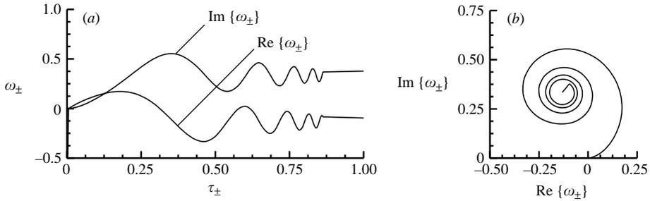
FIGURE 4. The solution for  $\omega_{\pm}(\tau_{\pm})$ ; (a) the real and imaginary parts of  $\omega_{\pm}(\tau_{\pm})$  plotted against the similarity variable  $\tau_{\pm}$ ; (b) a parametric plot of the self-similar spiral vortex sheet. In the case pictured above  $J_{\pm} \approx -6.4352$ .
