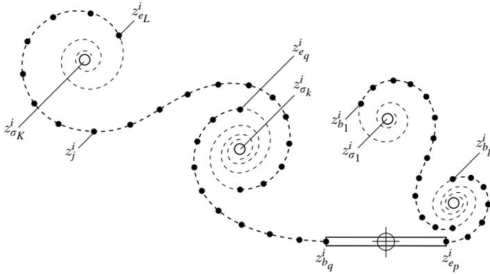
FIGURE 5. The discretized vortex wake in the body frame. The trailing vortex sheets are discretized using  $J$  Lagrangian vortex blobs ( $\bullet$ ), any tightly wound spiral portions being replaced with a point vortex at the spiral centre ( $\circ$ ). In total, there are  $K$  point vortices and  $L$  vortex blob sheets.
