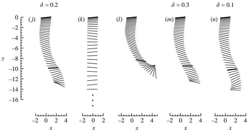
FIGURE 17. Examples (j)–(n). The trajectories of a falling flat plate after its release from rest with  $Fr = 4$  and  $\theta_0 = \pi/32$ . The wake is modelled as (j) two regularized vortex sheets with  $\delta = 0.2$ , (k) no wake, (l) a pair of point vortices, (m) two regularized vortex sheets with  $\delta = 0.3$ , and (n) two regularized vortex sheets with  $\delta = 0.1$ . The plate positions at  $t = 16$  are highlighted.
