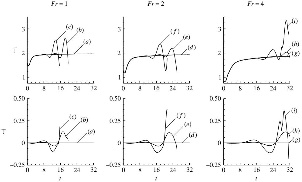
FIGURE 14. The aerodynamic normal force and torque on a falling plate after release from rest; examples (a)–(i). The functions  $\mathbb{F}(t)$  and  $\mathbb{T}(t)$  are plotted for modified Froude numbers (a)–(c)  $Fr = 1$ , (d)–(f)  $Fr = 2$ , and (g)–(i)  $Fr = 4$  and initial angles (a)(d)(g)  $\theta_0 = 0$ , (b)(e)(h)  $\theta_0 = \pi/1024$ , and (c)(f)(i)  $\theta_0 = \pi/256$ .
