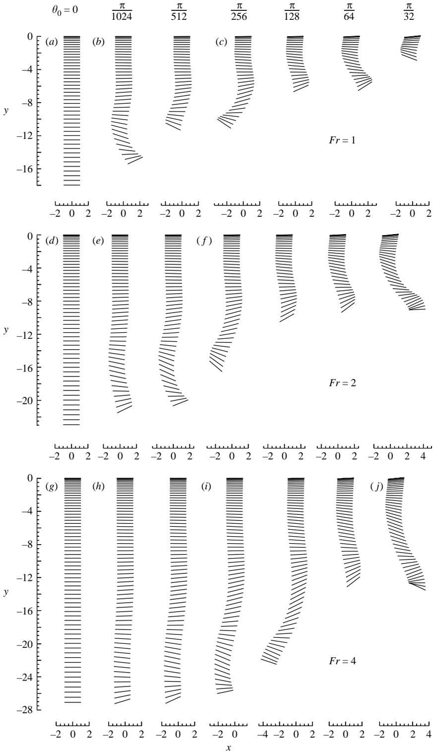
FIGURE 6. The trajectories of a falling flat plate after its release from rest. The trajectories are shown for  $\theta_0 = 0, \pi/1024, \pi/512, \pi/256, \pi/128, \pi/64$ , and  $\pi/32$  for each of the three modified Froude numbers  $Fr = 1, 2$ , and  $4$ . The labelled trajectories are discussed further in the text.
