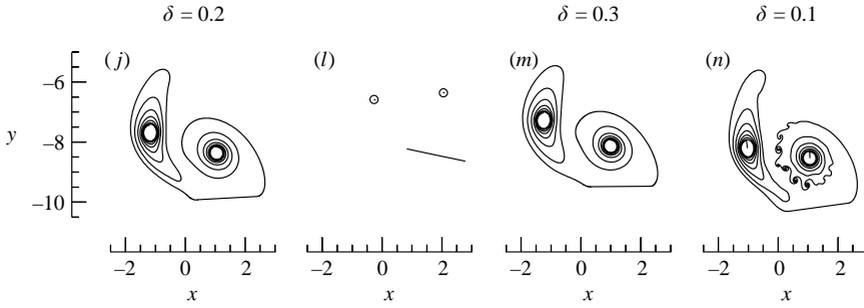
FIGURE 18. Examples (j), (l), (m), and (n). The wake behind a falling flat plate at  $t = 16$  after its release from rest with  $Fr = 4$  and  $\theta_0 = \pi/32$ . The wake is modelled as (j) two regularized vortex sheets with  $\delta = 0.2$ , (l) a pair of point vortices, (m) two regularized vortex sheets with  $\delta = 0.3$ , and (n) two regularized vortex sheets with  $\delta = 0.1$ .
