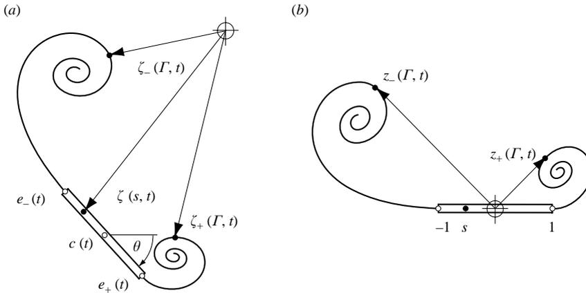
FIGURE 2. The dependent variables in (a) the rest frame of the fluid in the far field and (b) the body frame. The centre of the plate  $c(t)$ , the orientation angle  $\theta(t)$ , the plate edges  $e_{\pm}(t)$ , the position of a point on the plate  $\zeta(s, t)$ , and the position of a point on the shed vortex sheets  $\zeta_{\pm}(\Gamma, t)$  (or  $z_{\pm}(\Gamma, t)$  in the body frame).
