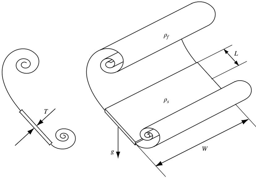
FIGURE 1. A cross-section and three-dimensional diagram of the falling plate and its vortex wake indicating the plate thickness  $T$ , half-chord  $L$ , width  $W$ , plate density  $\rho_s$ , fluid density  $\rho_f$  and the gravitational field strength  $g$ .
